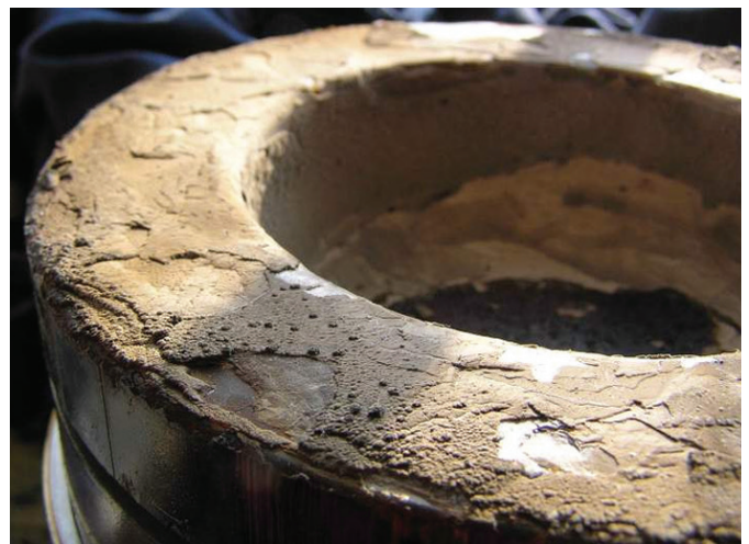
Figure 1. Severe deposits originating from siloxanes on the piston crown.
