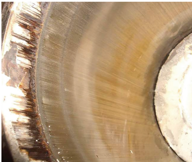
Figure 2. Abrasive wear caused by silicon dioxide deposits ground between rings and liner.
