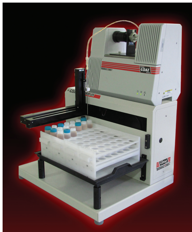
Figure 1. COAT system used for the FTIR determination of ASTM-identical AN and BN results for in-use mineral oils.
